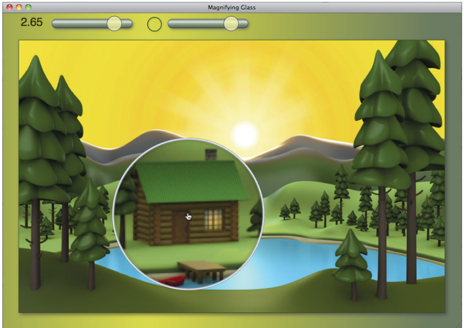
Figure 4.1 A magnifying glass that scales pixels and uses the clipping region
