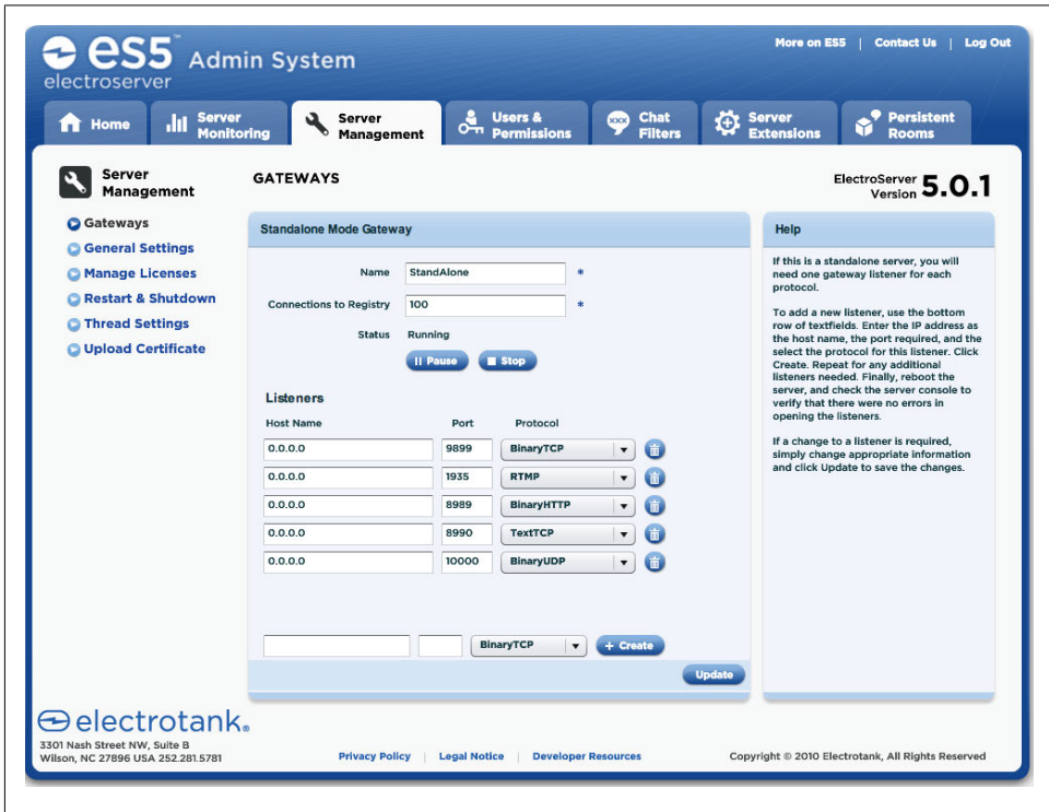
Figure 11-4. ElectroServer ports and protocols
