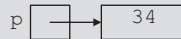
FIGURE 3-7 Pointer p and the value of the memory location to which p points
