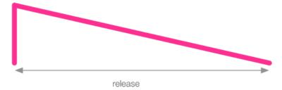
The vertical line at the far left of the diagram shows that the sound starts at 0 amplitude, but goes up to full amplitude immediately (this is the attack phase which we'll cover next). Once at full amplitude it then moves in a straight line down to zero taking the amount of time specified by release:. Longer release times produce longer synth fade outs.
