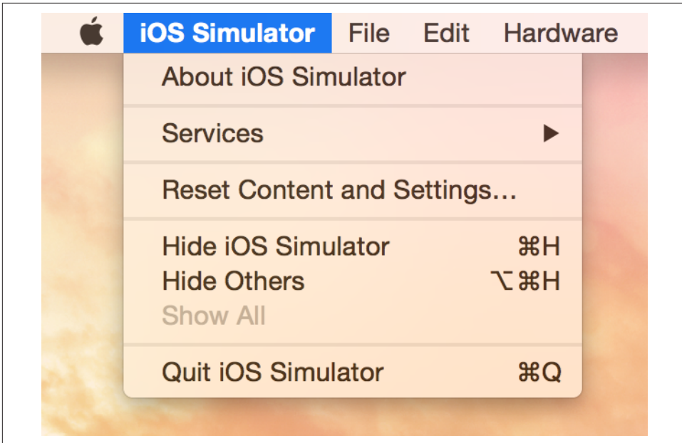
Figure 8-17. The Reset Content and Settings... option will delete everything from your device
