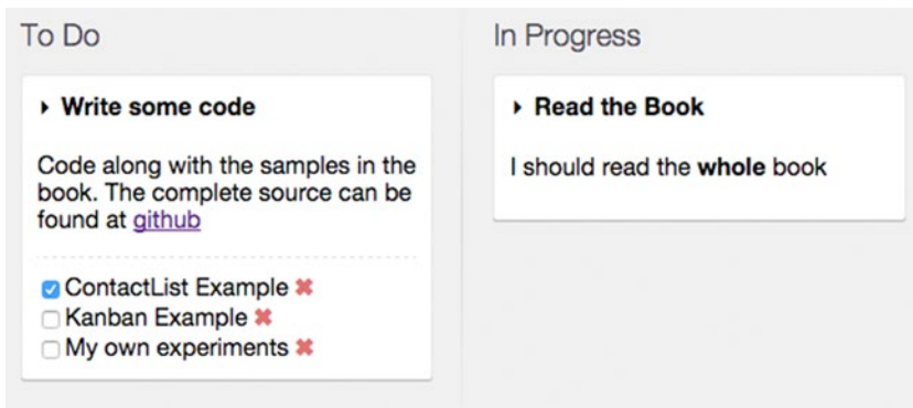
Figure 2-6. React rendering dynamically generated HTML with dangerouslySetInnerHTML
