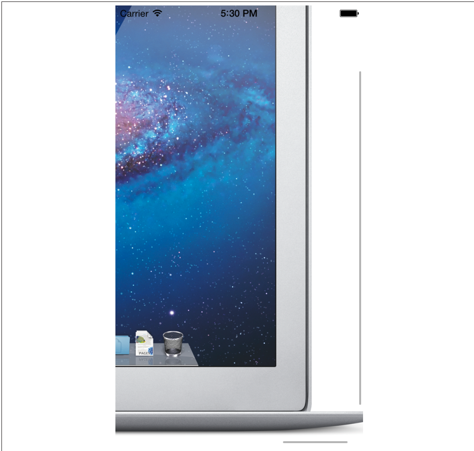
Figure 1-63. Black indicators appearing on the right and bottom of a scroll view
