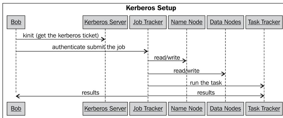
Kerberos setups will include a Hadoop cluster—NameNode, DataNodes, JobTracker, and TaskTrackers—and a Kerberos server. We will define users as **principals** in the Kerberos server. Users can obtain a ticket from the Kerberos server, and use that ticket to log in to any server in Hadoop. We will map each Kerberos principal with a Unix user. Once logged in, the authorization is performed based on the Unix user and group permissions associated with each user.
