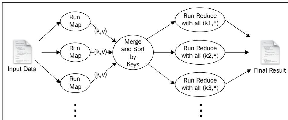
To run a MapReduce job, users should furnish a `map` function, a `reduce` function, input data, and an output data location. When executed, Hadoop carries out the following steps:
