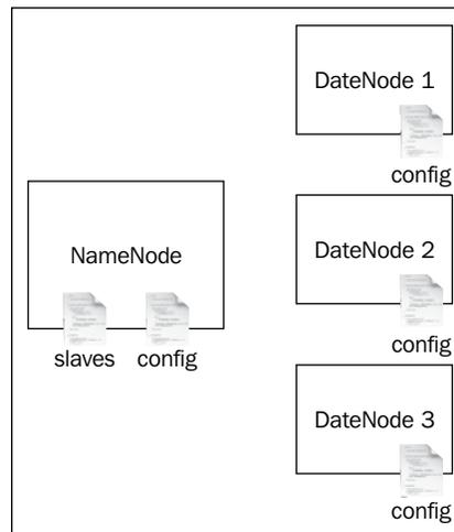
For the HDFS setup, we need to configure NameNodes and DataNodes, and then specify the DataNodes in the `slaves` file. When we start the NameNode, startup script will start the DataNodes.
