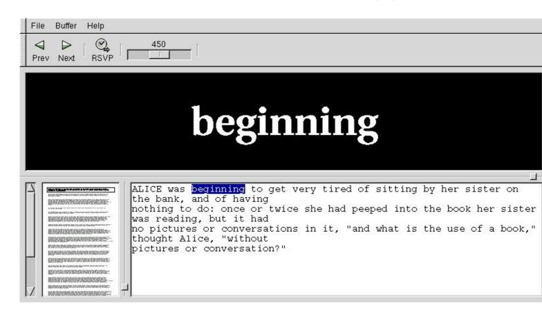
The large area with the word `beginning' in it is where the text is being streamed. The text in the lower—left window is a shrunken view of the entire file, the text in the lower—right window is the paragraph from which the current word comes from.
