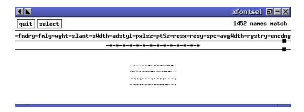
The row of buttons are pull—down menus containing options available on your system for each field in the X font name. Use the mouse to select items from each menu, and the X font you have selected is shown in the main window. Above it is written its X font name.
