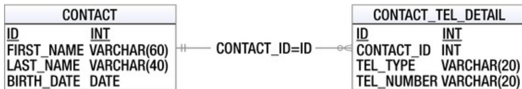
Figure 8-1. Simple data model for example code
