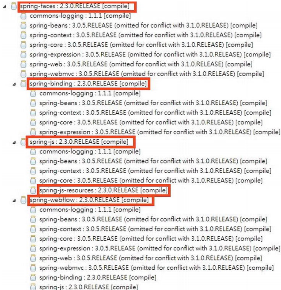
Figure 18-5. Dependency hierarchy of Spring Web Flow
