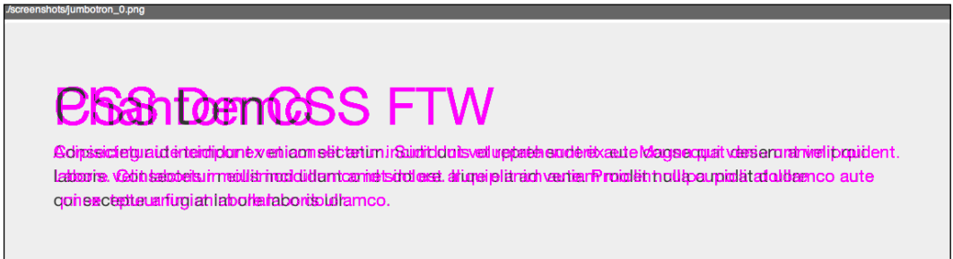
The image shows our failure diff and writes the image to disk as jumbotron_0.fail.png
