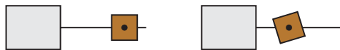
Figure 13.17 Groove joint: Object B moves and rotates along a groove on object A
