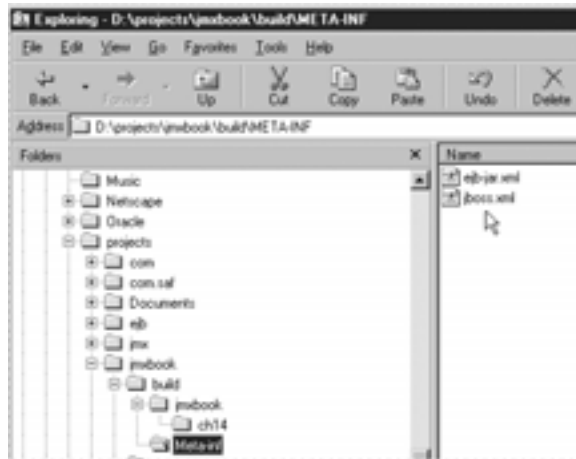
Figure 14.4 Directory structure under the build directory for deployment of the entity bean.
