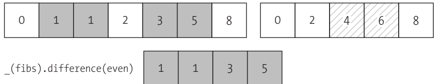
FIGURE 8-9: The difference() function returns elements that are present only in the first of multiple arrays.
