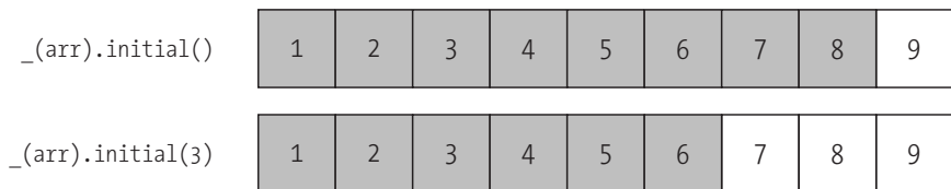
FIGURE 8-4: The initial() function returns all but the last element or all but the last n elements in an array.
