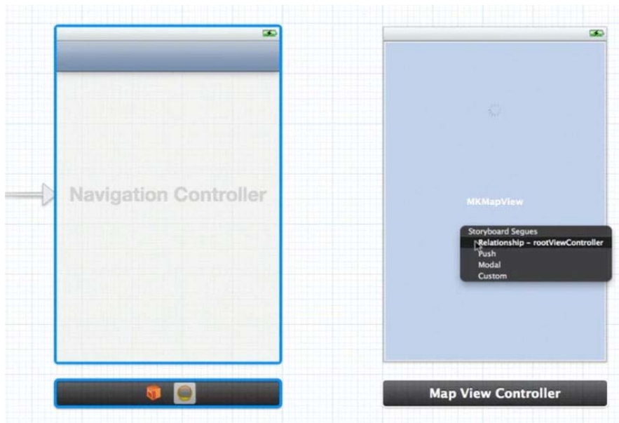
Figure 3-35. Create the rootViewController relationship.
