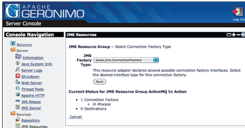
Figure 8.11 Easily create a JMS connection factory for ActiveMQ via the Geronimo console.
