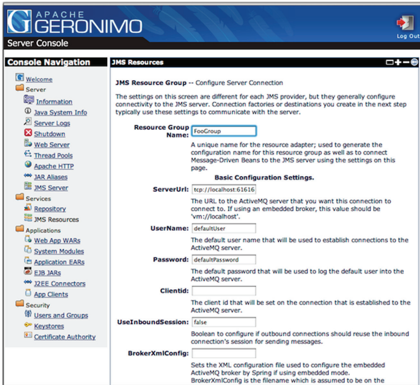
Figure 8.9 Accept the default values when configuring the ActiveMQ resource adapter's server connection.
