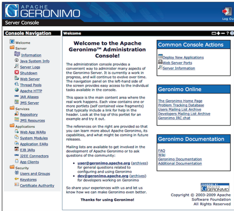
Figure 8.6 The Geronimo console provides the ability to manage ActiveMQ (the JMS Server) and the ActiveMQ resources (JMS Resources).
