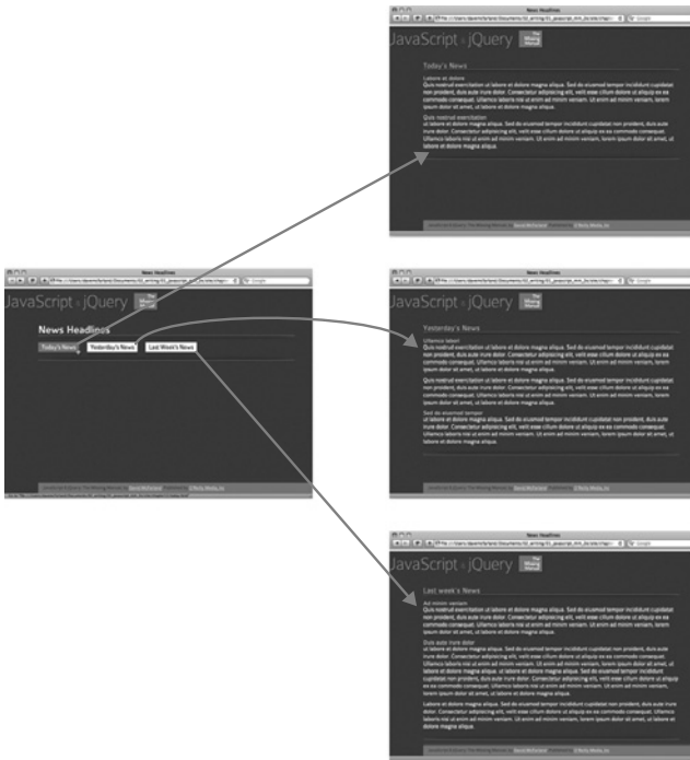
Figure 11-3: The top set of images shows how links work—the typical method of accessing additional HTML. Click a link on a page (top left) and it loads a brand new page (top right). However, using Ajax and jQuery's load() function, you can access the same HTML without leaving the current web page (bottom). Clicking a link loads the HTML content into a <div> tag (outlined).
