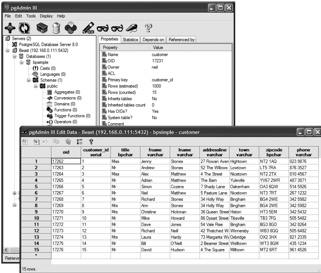
Figure 2-5. Viewing customer data from a database with pgAdmin III
