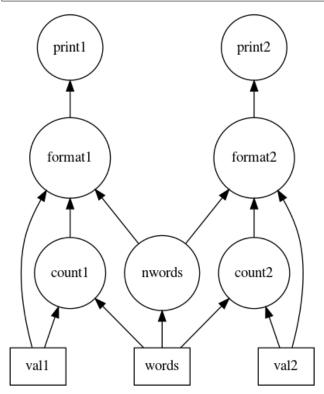
Looking at the task graph above, there are multiple accesses to constants such as 'vall' or 'vall' in the Dask graph. These can be inlined into the tasks to improve efficiency using the inline function. For example:
