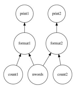
Now we have two sets of *almost* linear task chains. The only link between them is the word counting function. For cheap operations like this, the serialization cost may be larger than the actual computation, so it may be faster to do the computation more than once, rather than passing the results to all nodes. To perform this function inlining, the inline\_functions function can be used:
