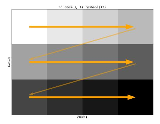
Now consider the impact of Dask's chunking on this operation. If the slow-moving axis (just axis=0 in this case) has chunks larger than size 1, we run into a problem.
