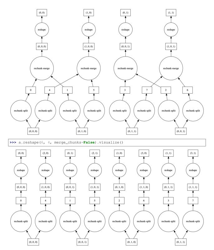
By default, some intermediate chunks chunks are merged, leading to a more complicated task graph. With merge\_chunks=False we split the input chunks (leading to more overall tasks, depending on the size of the array) but avoid later communication.
