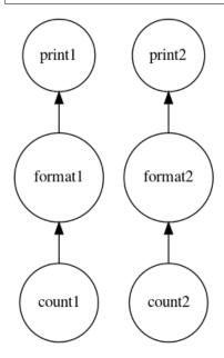
Now we have a set of purely linear tasks. We'd like to have the scheduler run all of these on the same worker to reduce data serialization between workers. One option is just to merge these linear chains into one big task using the fuse function:
