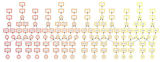
At a glance, we can see that this ordering is looks much more regular and uniform. There's fewer lines crossing, and the color of the ordering moves smoothly from bottom to top, left to right. This shows that Dask is completing one chain of computation before moving onto the next.
