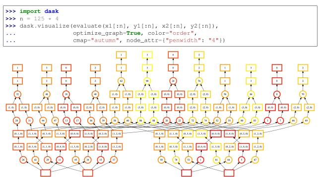
In this visualization the nodes are colored by order of execution (from dark red to light yellow) and the node labels are the order Dask's assigned to each task.
