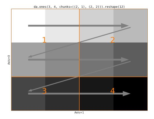
The first block has a shape (2, 2). Following the rules of reshape we take the two values from the first row of block 1. But then we cross a chunk boundary (from 1 to 2) while we still have two "unused" values in the first block. There's no way to line up the input blocks with the output shape. We need to somehow rechunk the input to be compatible with the output shape. We have two options
